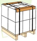
It is used to protect the packaging aganist straping damages
